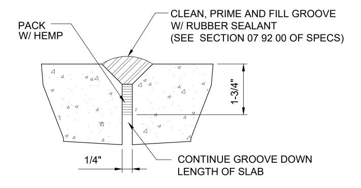
SEALANT GROOVE DETAIL NOT TO SCALE PL-05-3 071003
