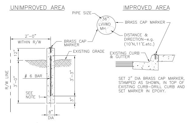
SET 2" DIA BRASS CAP MARKER STAMPED AS SHOWN, IN 8" DIA REINFORCED CONCRETE.
