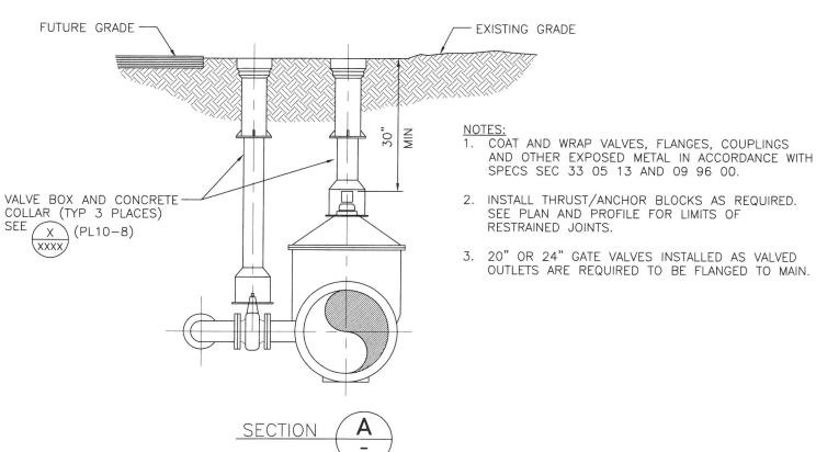
20" AND 24" DIRECT BURIED GATE VALVE WITH BY-PASS INSTALLATION (DIP)
