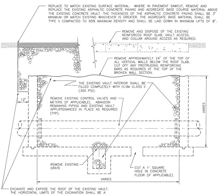
THE HORIZONTAL LIMITS OF THE EXCAVATION SHALL BE A MINIMUM OF 12" GREATER ON ALL SIDES AND 30" BELOW THE TOP OF THE EXPOSED VAULT STRUCTURE.
