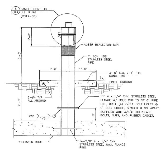
FOR EXISTING RESERVOIR INSTALLATION, CUT & REMOVE EXISTING 6" SAMPLE PORT PIPE AS SHOWN. WELD 11" Ø x 1/4" THK. STAINLESS STEEL FLANGE W/HOLE CUT TO FIT EXISTING 6" PIPE O.D., DRILL (4) 7/8"Ø BOLT HOLES @ 9" BOLT CIRCLE SPACED @ 90' APART TO MATCH NEW 6" SAMPLE PORT FLANGE.
