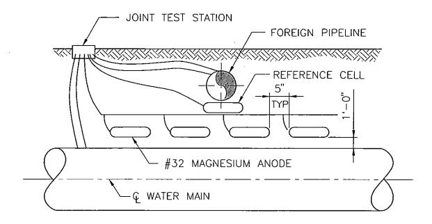
ATTACH ANODE LEAD WIRE TO COLLECTOR CABLE WITH THOMAS ASN BETTS "C" CRIMP OR EQUAL. SEAL SPLICES WITH AQUARIAL AND ELECTRICAL TAPE OR EQUAL. LEAVE SUFFICIENT SLACK IN CABLE FOR TERMINATION AND TO RELIEVE STRESS ON WIRE DURING BACKFILL
