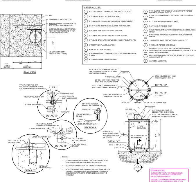
AIR VALVE ASSEMBLY FOR 2-INCH AND 4-INCH VALVES
